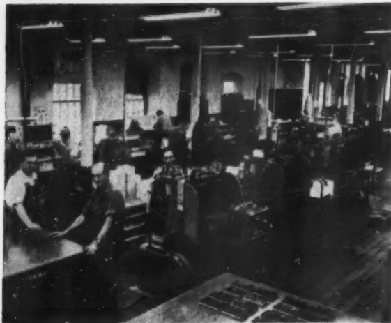
Six Miehle Vertical Presses have been placed in two opposing rows in plant of Excelsior Printing Co., North Adams, Mass., with 20 ft. long work table between. The presses are operated by a crew of four men. See accompanying story in which is explained how maximum production is secured.
